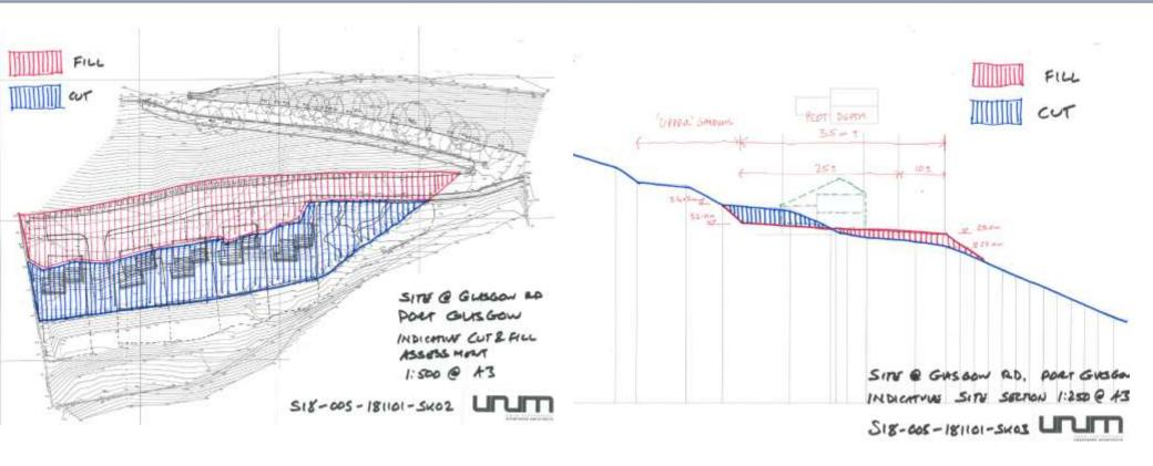
5.2.2 & 5.2.3 Sketch site plan and section showing layout plan and estimated extent of cut and fill required
